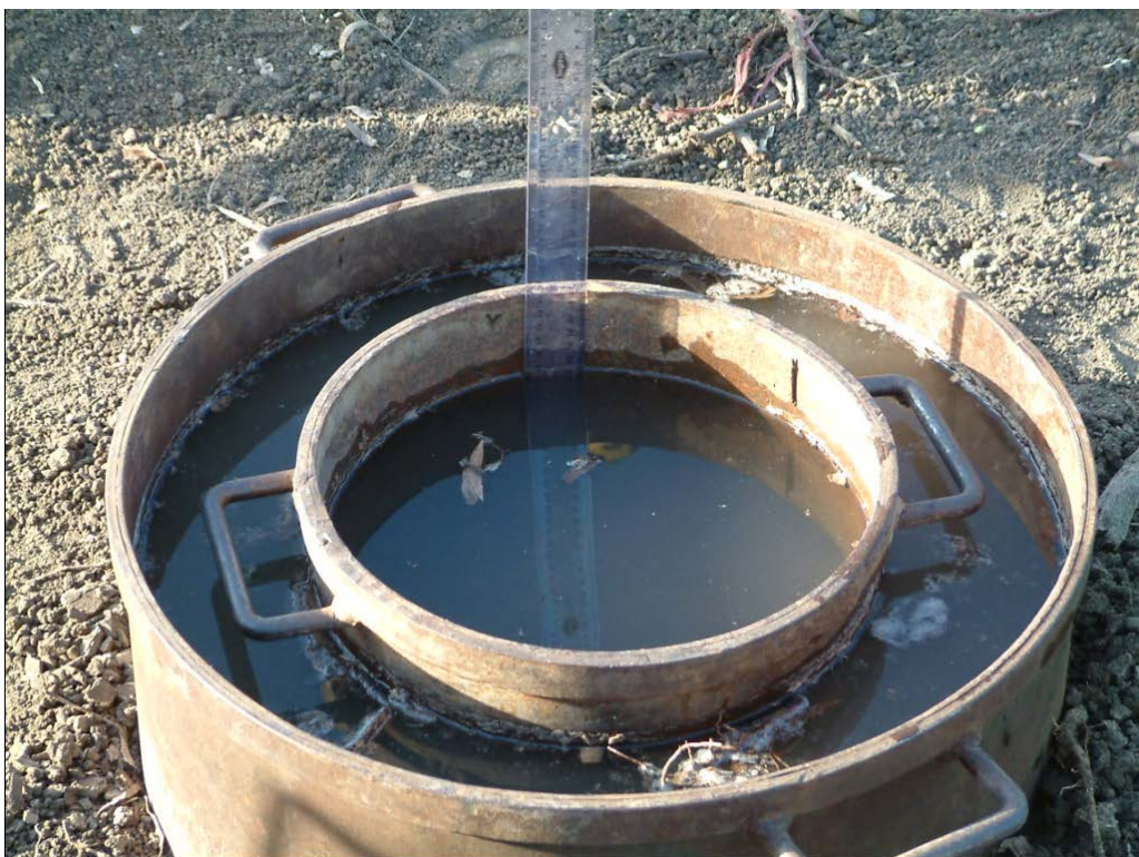
Photo 2 – Simple Double Ring Infiltrometer
