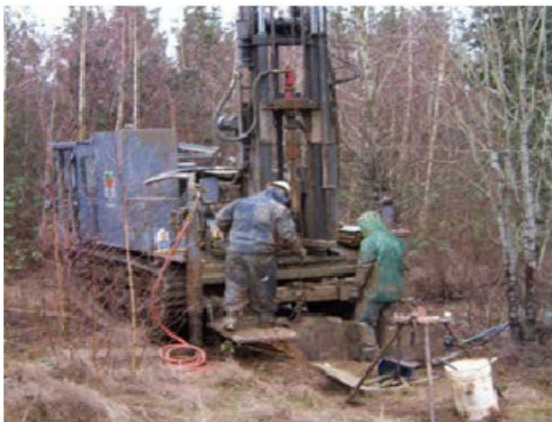
Photo 8- Auger Boring Rig
